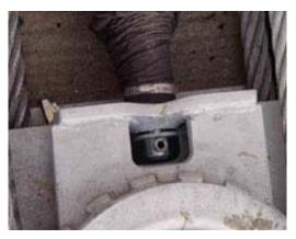
The cylinder rod pushed the ½" plate back ½" but did not fail. Our units have been impacted numberous times at 75 mph and this plate has never fatigued but with an impact that was 2.3 times above NCHRP350 criteria, it still held.
