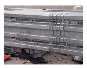
Incident above was impacted at very high speed. The ¾ ton pickup was making a quick change from an HOV lane into regular traffic. The vehicle hit the attenuator just left of center in front of the steering wheel.
